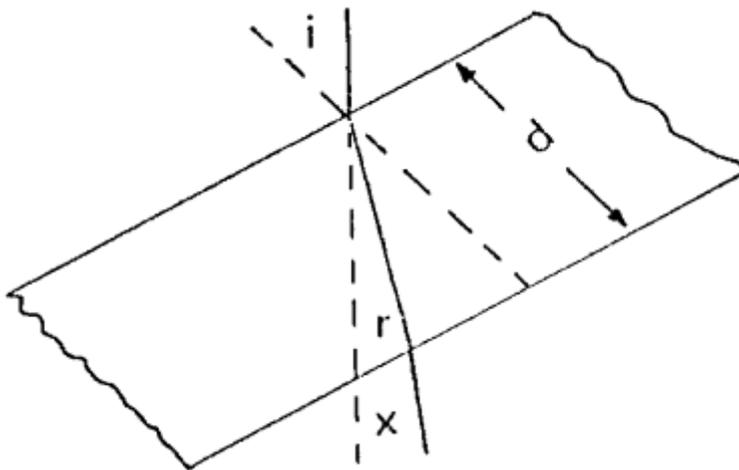
Figure 1 Glass "prism" refractive index  $n$ , thickness  $d$ .
