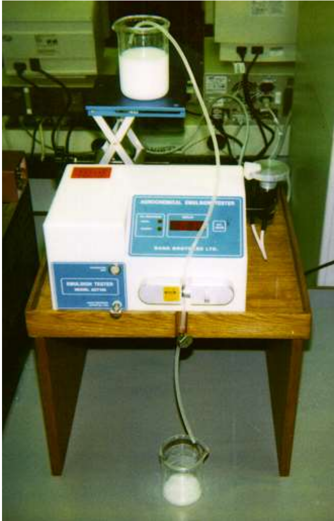
Figure 4 The Agrochemical Emulsion Tester (AET100).
